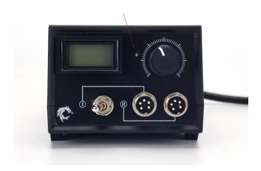
As you turn the knob, the voltage will increase by an increment of 2. Once the knob is turned half way (the middle setting), your device will be showing approximately 120 to 130V and the wire tip might start glowing. We DO NOT recommend going past the middle setting as it might make the pen itself heat up and become too hot to touch.
